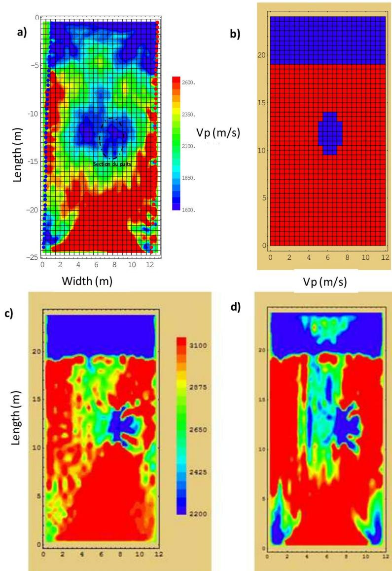
Figure 2 : Example results of mine shaft exploration using seismic tomography
