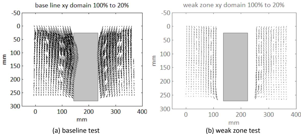
Figure 14 : Displacement of soil around shaft when shaft internal air pressure reduced to 20% of its original value for (a) baseline test, and (b) weak zone test.
