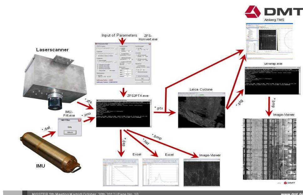
Figure 3: Workflow of data processing
