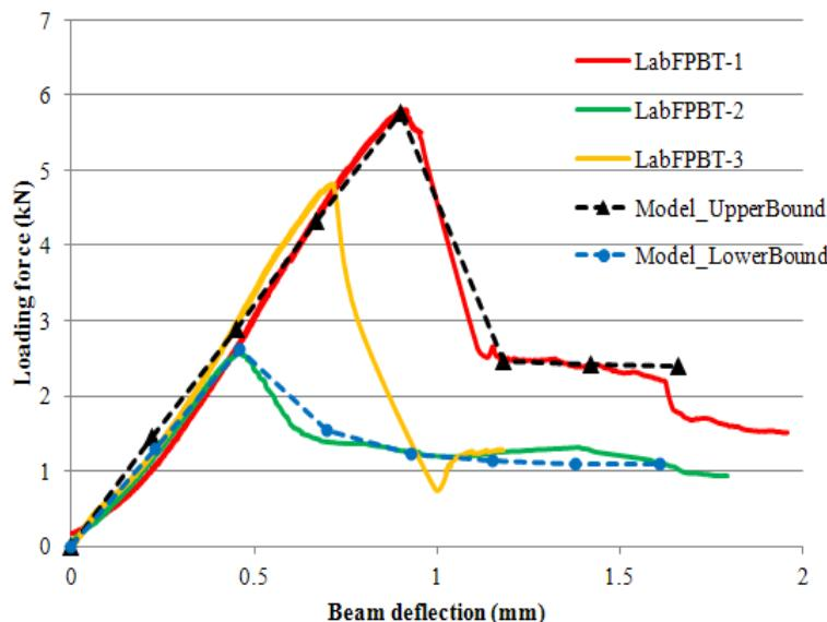
Figure 10 : Force-deflection curves for FPBT on brickwork beam from numerical models & laboratory tests
