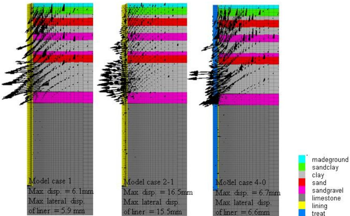
Figure 11 : Displacement vectors of Model case 1, 2-1 and 4-0
