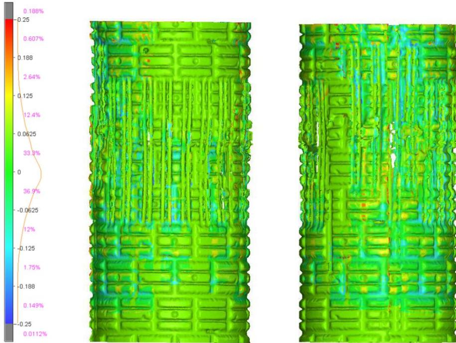
Figure 6: Test of a local deformation analyses between two campaigns
