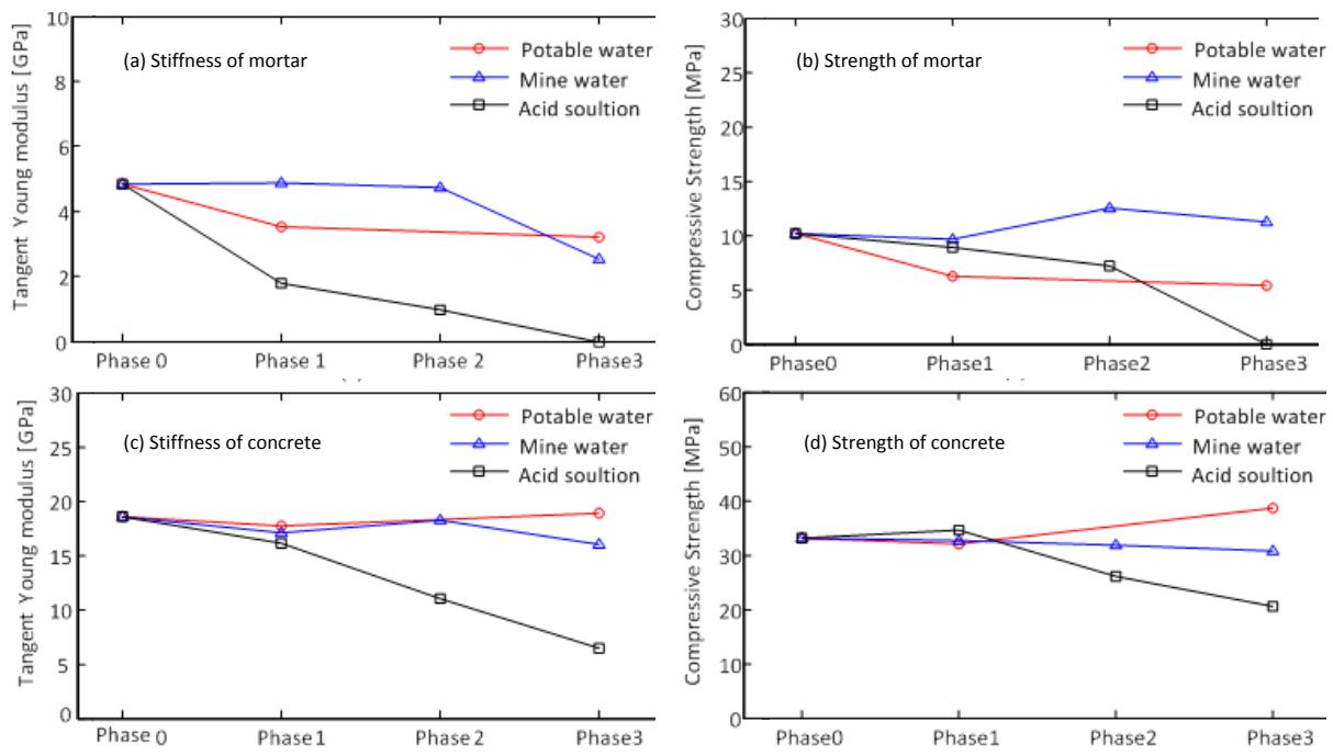
Figure 9 : UCS results for stiffness and strength change of concrete and mortar due to weathering
