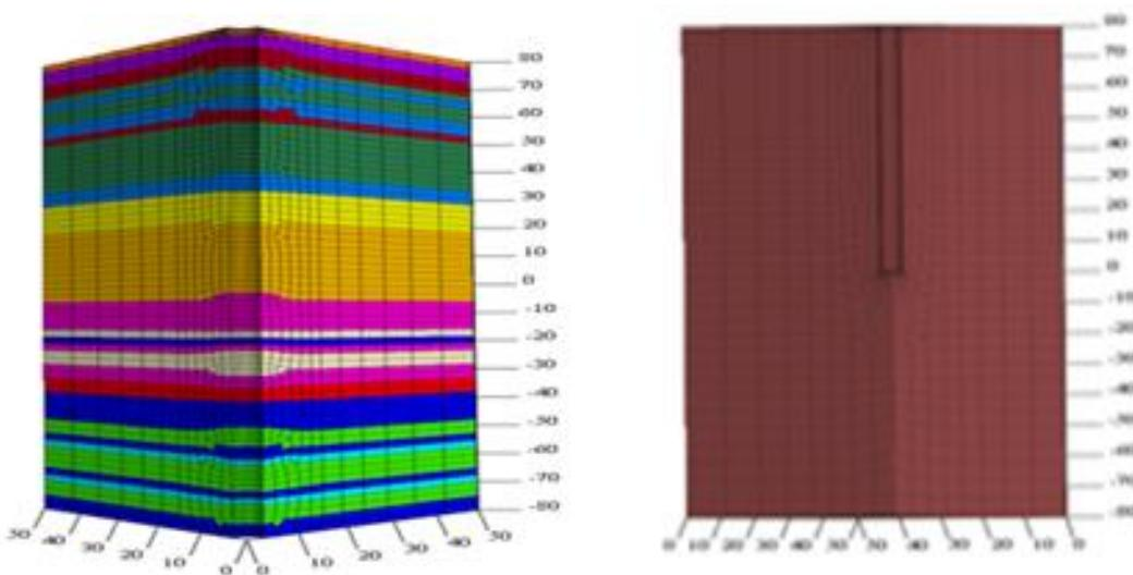
Figure 12 : Cross section of both models with geological properties (Model 1: Multicolor; Model 2: Brown)
