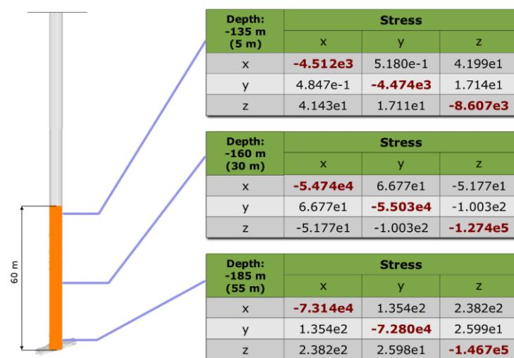
Figure 21 : An example of the state of stress in the three selected points in the filling column (MPa)
