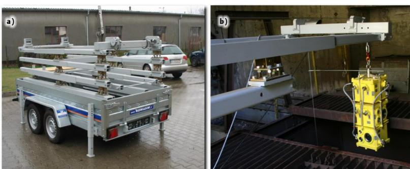
Car trailer is equipped with depth-encoders, WIFI antenna and special jibs enabling precise guidance of the probe anywhere in the area of the shaft.
