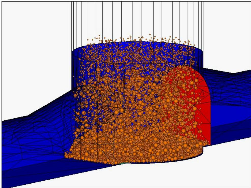
Figure 18 : Example of generated material with a defined grain size distribution and other physical properties (density, friction coefficient)
