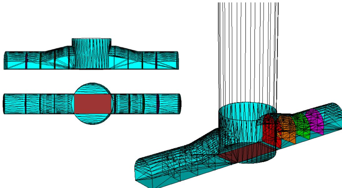
Figure 17 : View of the imported insets geometry with the variable location of the dams at level 190 m
