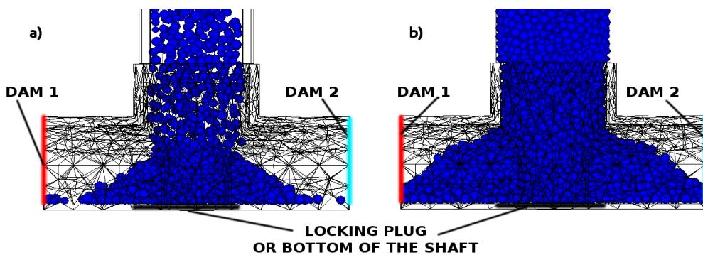
Figure 19 : Sequential stages of simulation of shaft filling – mouth view in shaft insets area.
