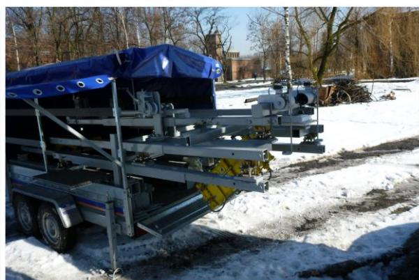
**Car trailer with probe mounted for transport**
