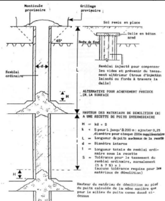
Principle of controlled back-filling of a mine shaft (National Coal Board, 1982).
