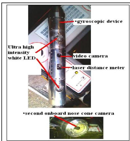
**Camera for flooded voids (probe 4)**
