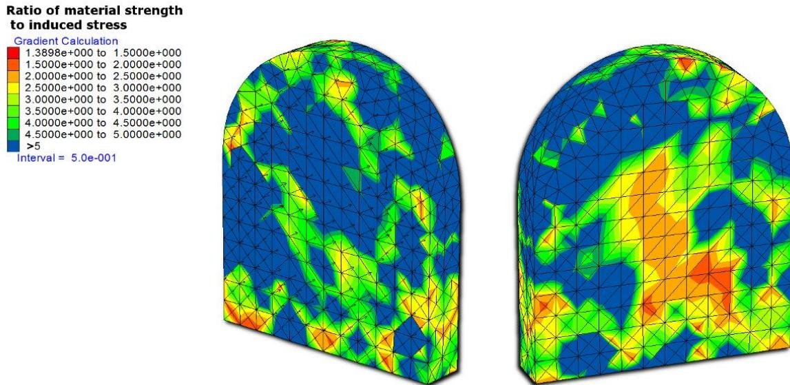
Figure 22 : Example of strength analysis using FLAC3D based on results from PFC3D
