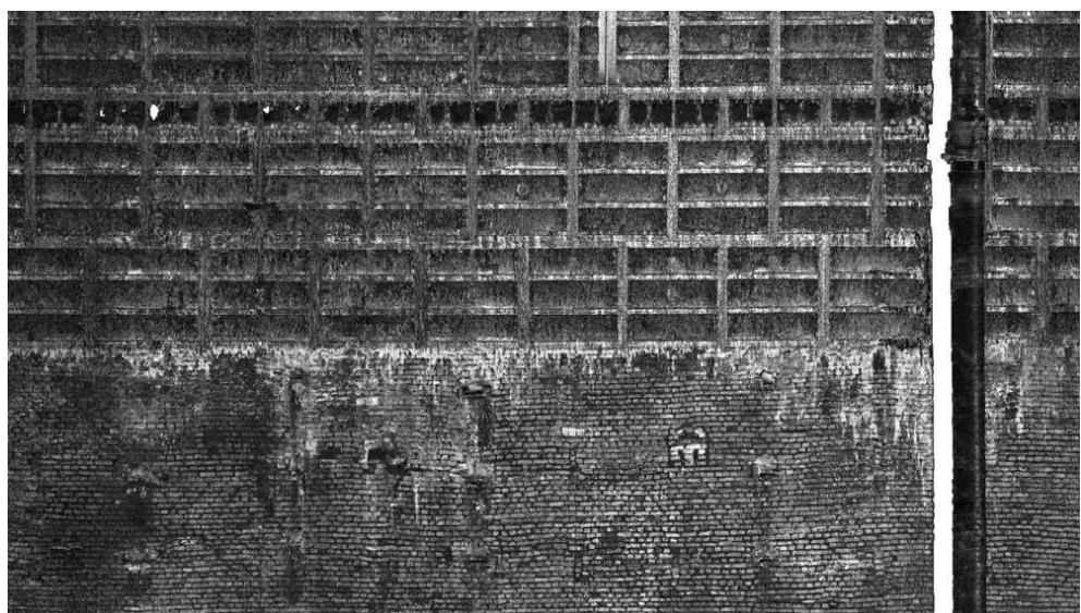
Figure 5: Unwrapped image of scan data (transmission from tubing to brick lining)
