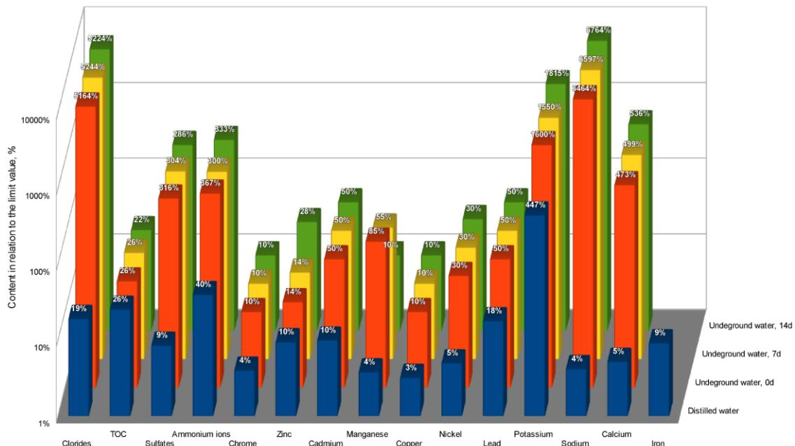
Figure 8 : Percentage of measured values in reference to acceptable values for blast furnace slag
