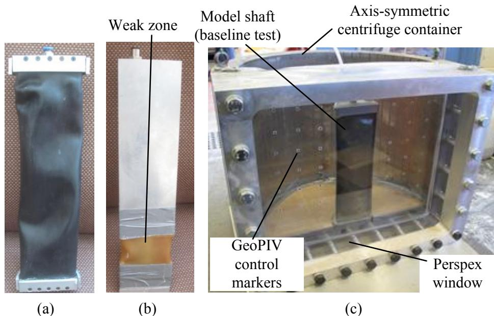
Figure 13 : (a) baseline test shaft, (b) weak zone shaft, (c) view of axis-symmetric container with baseline test shaft
